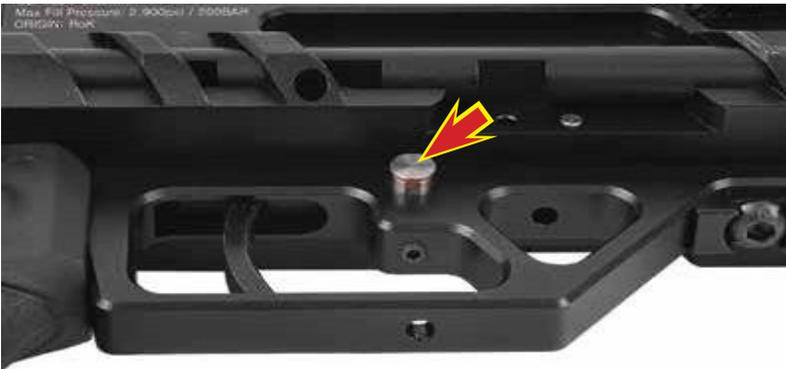
**In addition to the safety catch, a loaded and cocked rifle can be made safe by decocking (uncocking). To decock the rifle, first pull the sidelever back to the rear position and remove the magazine. While holding the sidelever, squeeze the trigger and let the lever return forward under your control. The rifle is now decocked.**
